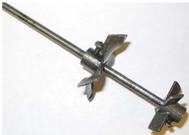
Fig. 6 Modified impeller shaft of Parr reactor
